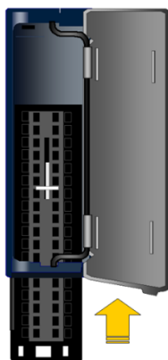
Figure 10: Slide FTB Terminal Block into Place
