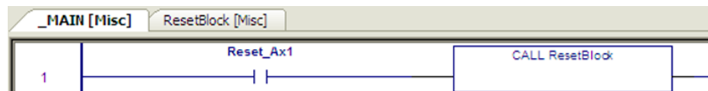
Figure 72: Resetting an Axis - Method Recommended
